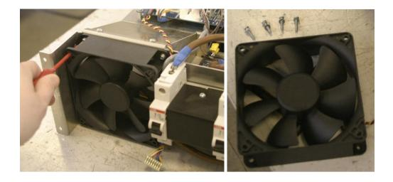
Retract the sheathing from the old fan wires, and unsolder them from the board.
