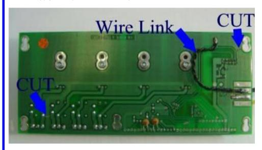
5. Solder the supply cables (yellow and black) as shown in top photo. Note that the 0V supply cable is on the pad directly above the wire link.
